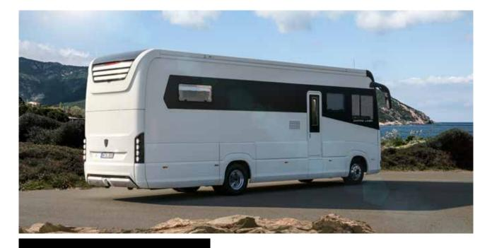
TECHNICAL SPECIFICATIONS (excerpt) Chassis: Iveco Daily Engine | Power: 3.0 L | 205 metric HP Gross weight: 7,490 kg Chassis: Mercedes Benz Atego Engine | Power: 7.7 L | 238 / 299 metric HP Gross weight: 9,500 – 15,000 kg
